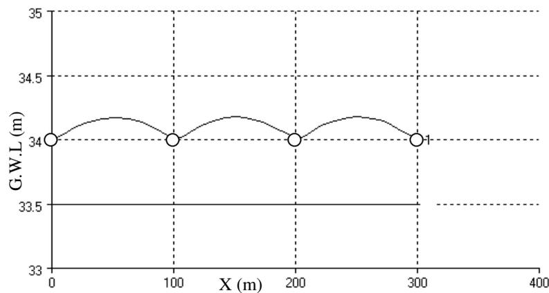
Figure 6: Water table profile at section (A-A) with perforated pipes
