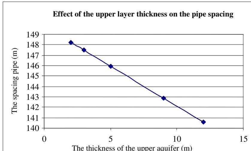
Figure 7: The effect of the upper layer thickness on the pipe spacing
