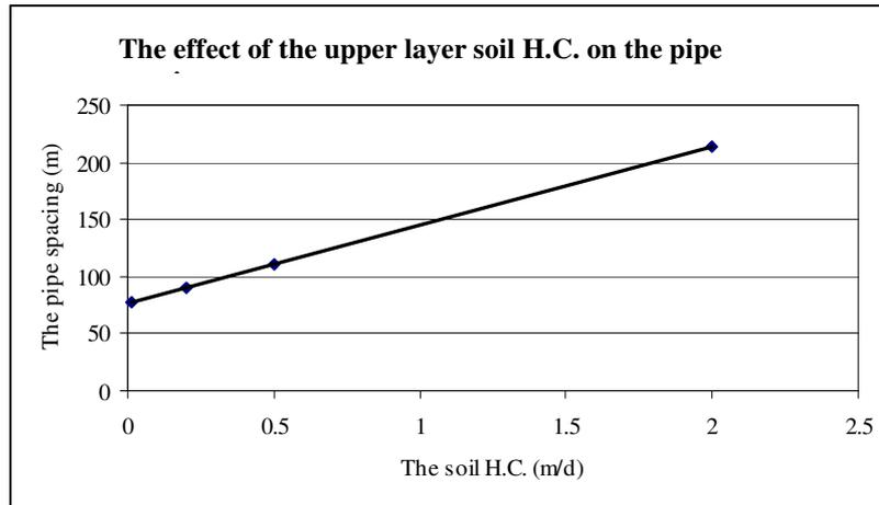
Figure 9: The effect of the upper layer soil H.C. on the pipe spacing
