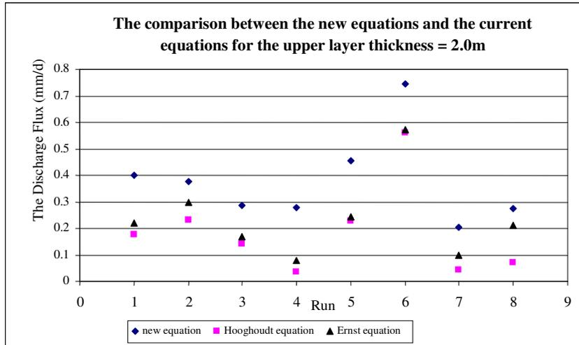
Figure (15): The comparison between the new equations and the current equations for the upper layer thickness of 2.0m
