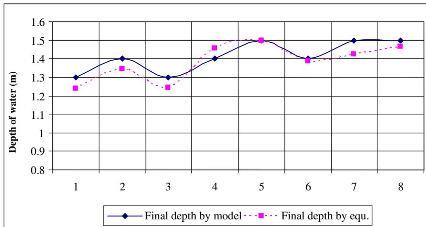
Figure (16): The comparison between the final depth of water in model and the final depth from the equation
