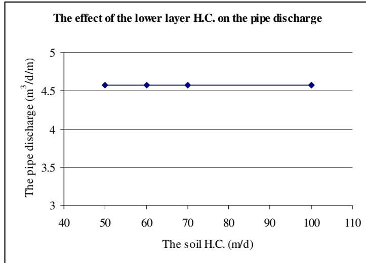
Figure 13: The effect of the lower layer soil H.C. on the pipe discharge
