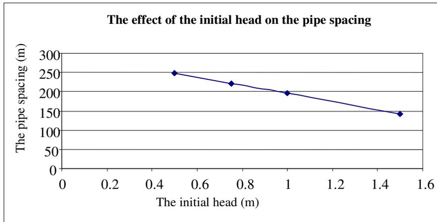
Figure 11: The effect of the initial head on the pipe spacing
