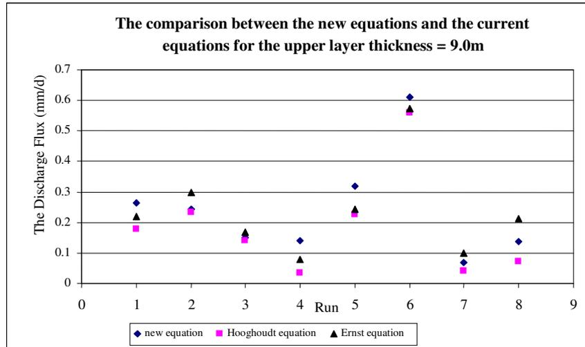
Figure (14): The comparison between the new equations and the current equations for an upper layer thickness of 9.0m
