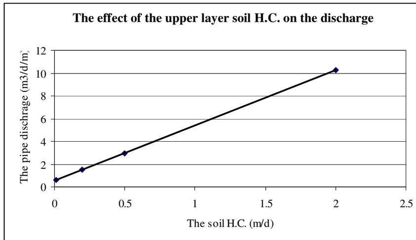
Figure 10: The effect of the upper layer soil H.C. on the pipe discharge
