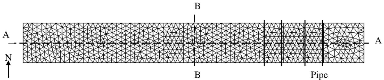
Figure 3: Finite Element Mesh for the numerical model
