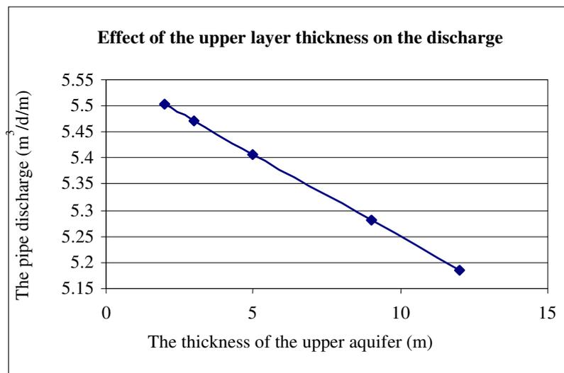
Figure 8: The effect of the upper layer thickness on the pipe discharge
