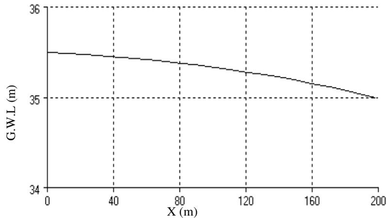
Figure 5: Water table profile at section (B-B) without perforated pipes
